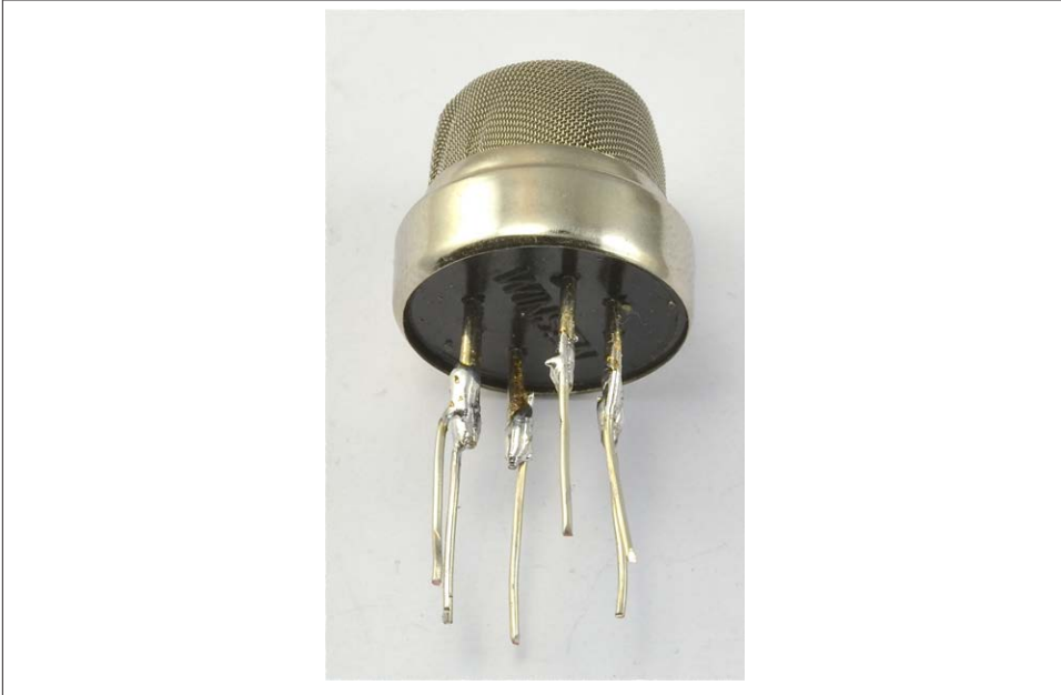
Figure 12-5. Soldering leads onto the gas sensor
