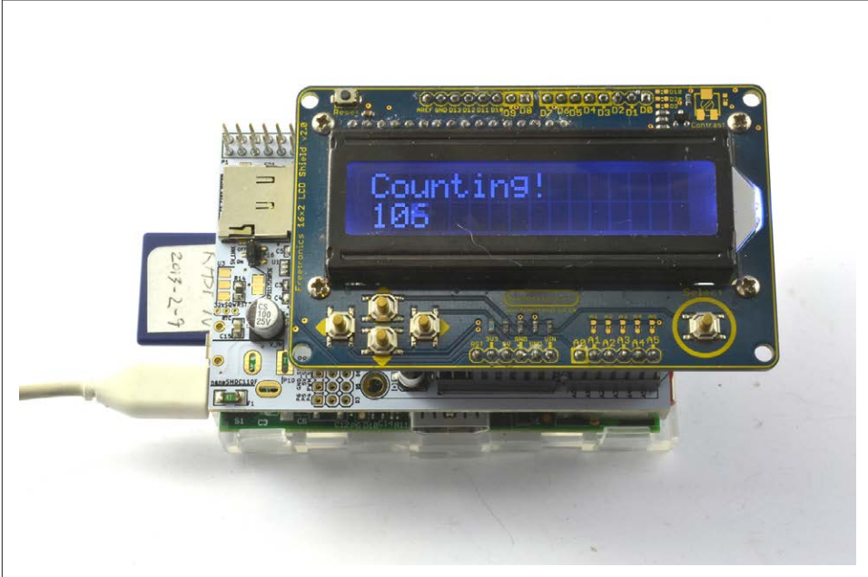
Figure 14-21. Using an LCD Arduino shield with an aLaMode
