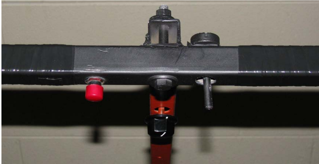
Figure 11-27. The large Red button on the left side of the handlebar is used as the Engage switch.
