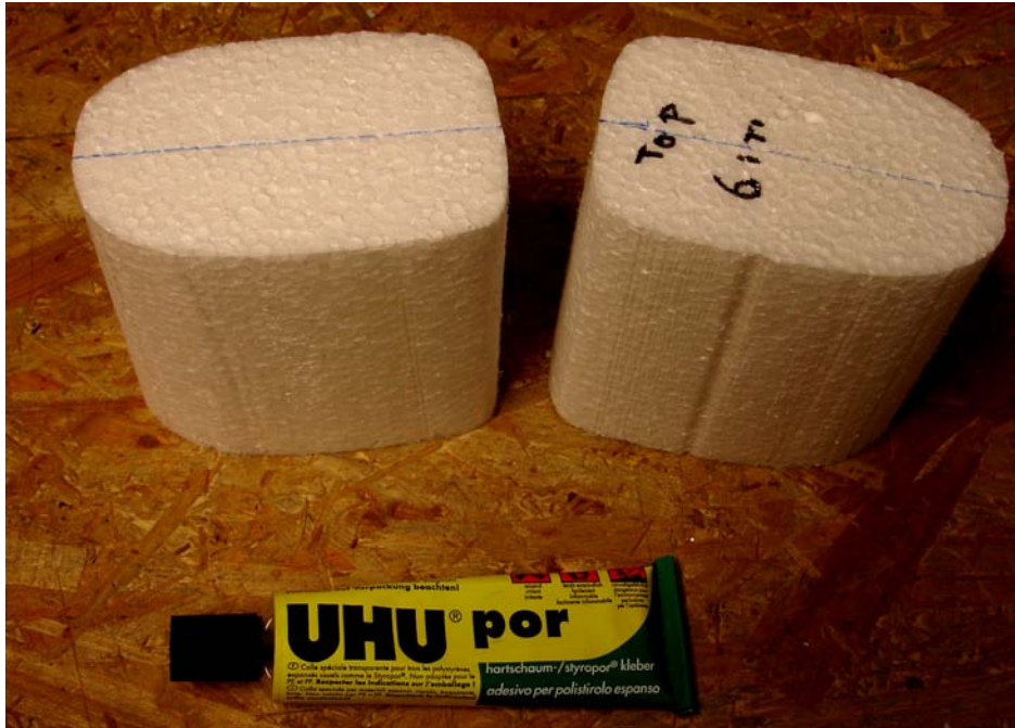
Figure 9-13. Two adjacent segments with EPS/XPS glue
