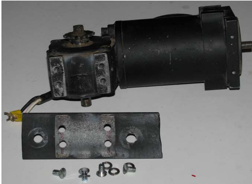
Figure 10-13. The motor mounting plate with 1/4-inch bolts
