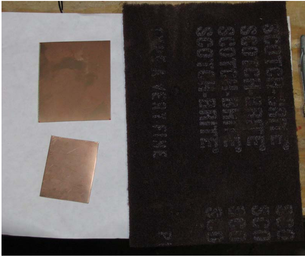
Figure 6-19. The two pieces of copper clad board cut to size and ready for cleaning
