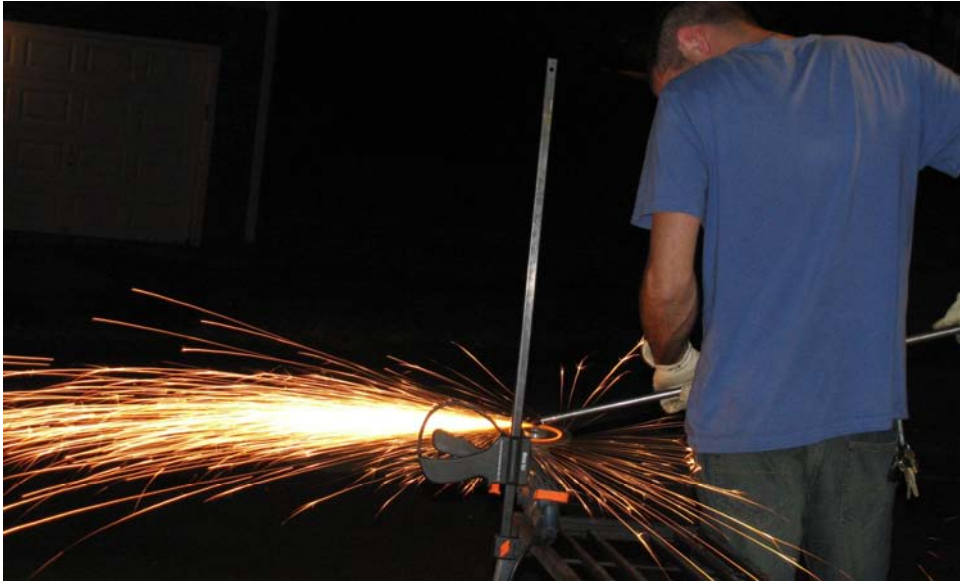
Figure 12-33. Grinding the spikes to make sharp points
