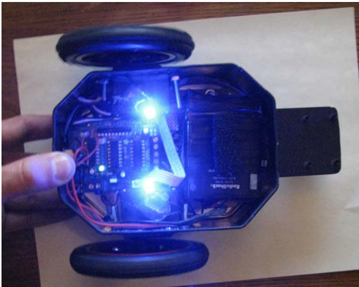
Figure 4-38. Both blue LEDs lit up as the bot is driving forward with both motors
