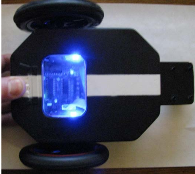
Figure 4-39. Both blue LEDs lit up with the lid on top—you can see through the plastic window.
