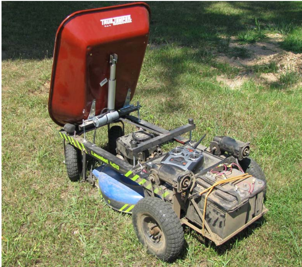
Figure 10-31. The Lawn-bot with dump bucket and linear actuator lift motor installed
