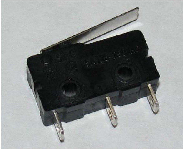
Figure 2-21. A typical tactile bump-switch with lever
