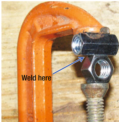
Figure 12-14. A C clamp holding the two nuts used to build the chain tensioning nut-assembly
