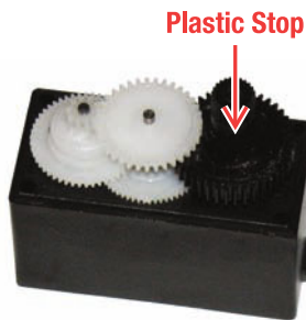
Figure 4-18. Using a soldering iron, melt away the plastic stop from the main black gear. It protrudes from the rest of the gear and keeps it from spinning continuously.
