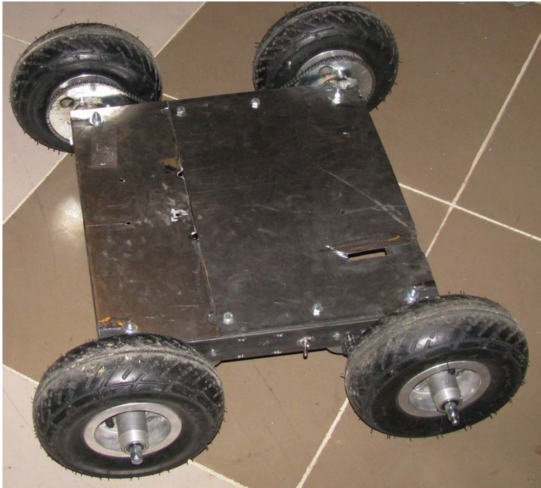
Figure 12-24. The basic frame fully assembled with armor
