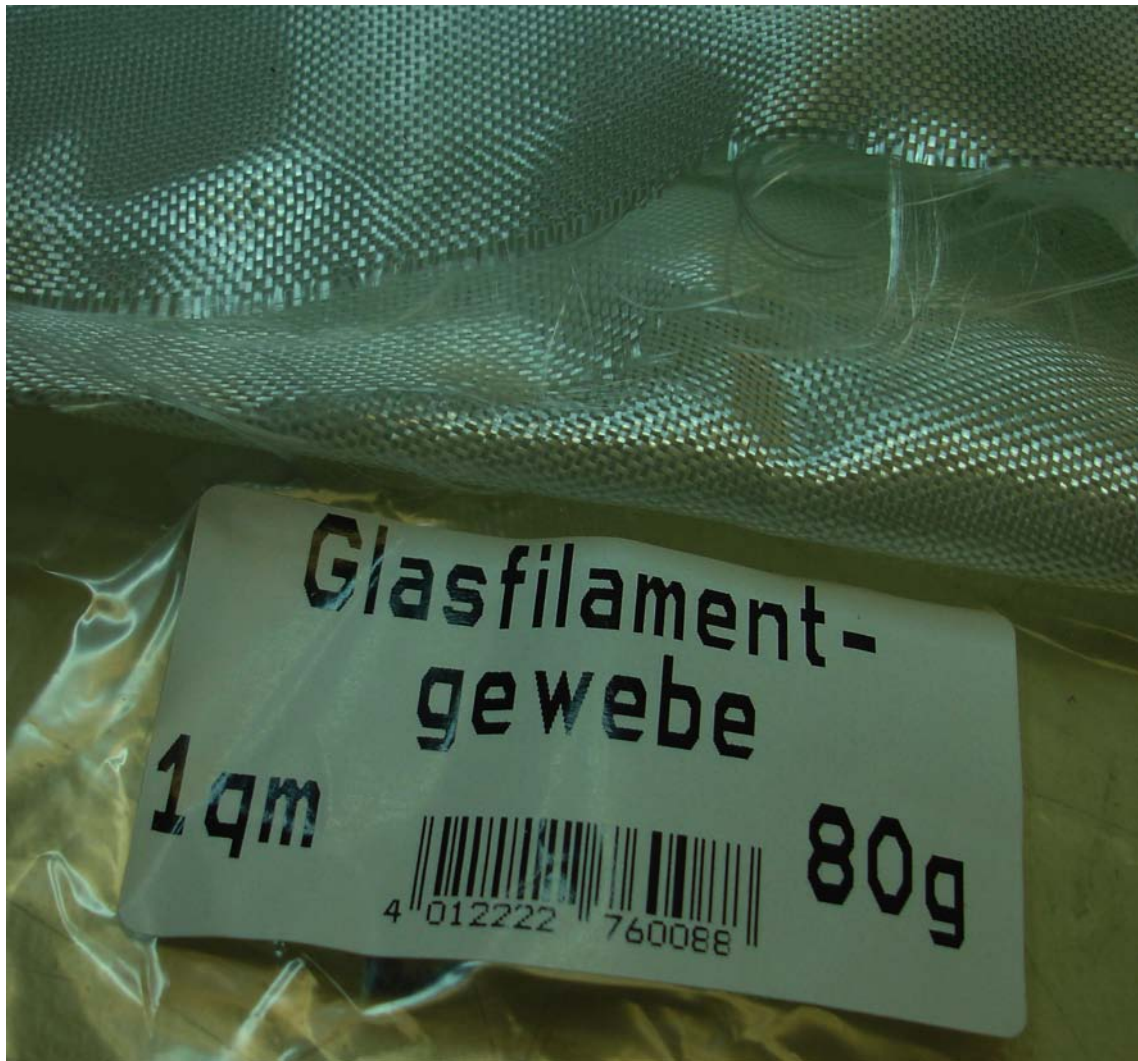
Figure 9-2. Woven fiberglass fabric with 80g/m 2
