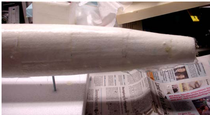
Figure 9-19. The hull, coated with fiberglass fabric and epoxy resin
