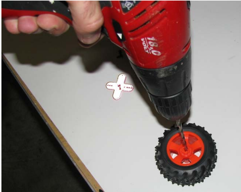
Figure 7-7. Drill the center of each wheel using a 1/4-inch drill bit to make a hole for the set screw to pass completely through, so the Servo output shaft set screw fits snugly against the Servo mounting plate.
