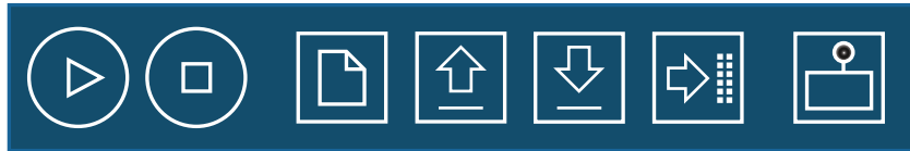
Figure 1-17. The IDE has a toolbar at the top that contains shortcuts for common tasks. You can hover your mouse cursor over each button when using the IDE to see a description.
