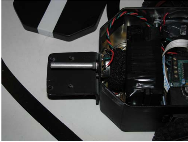
Figure 4-46. The speed control potentiometer mounted through the front of the frame
