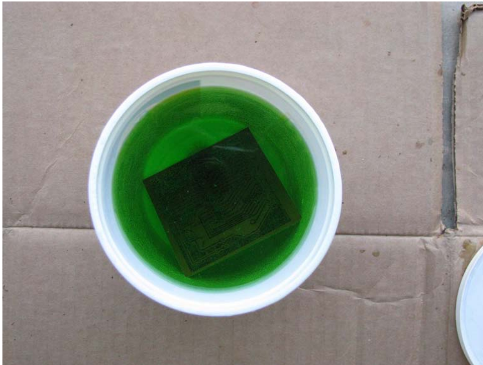
Figure 6-28. The plastic container with the PCB inside, about half-way finished etching
