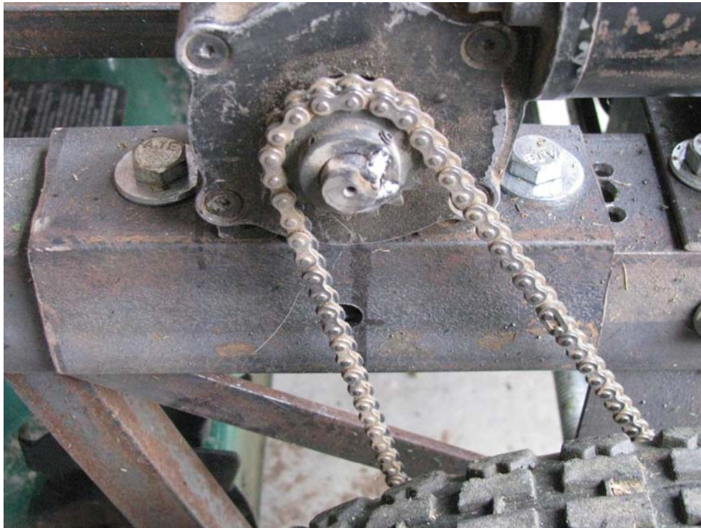
Figure 10-18. The motor with chain attached to both sprockets
