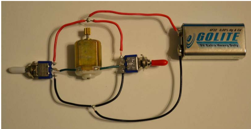
Figure 3-13. Here you can see a basic H-bridge circuit using two SPDT switches, a DC motor, and a 9v battery. Notice how the top terminals of each switch share a common positive supply wire, while the bottom terminals share a common negative supply wire. The center terminals of each switch are used to route the power signals to the motor terminals.
